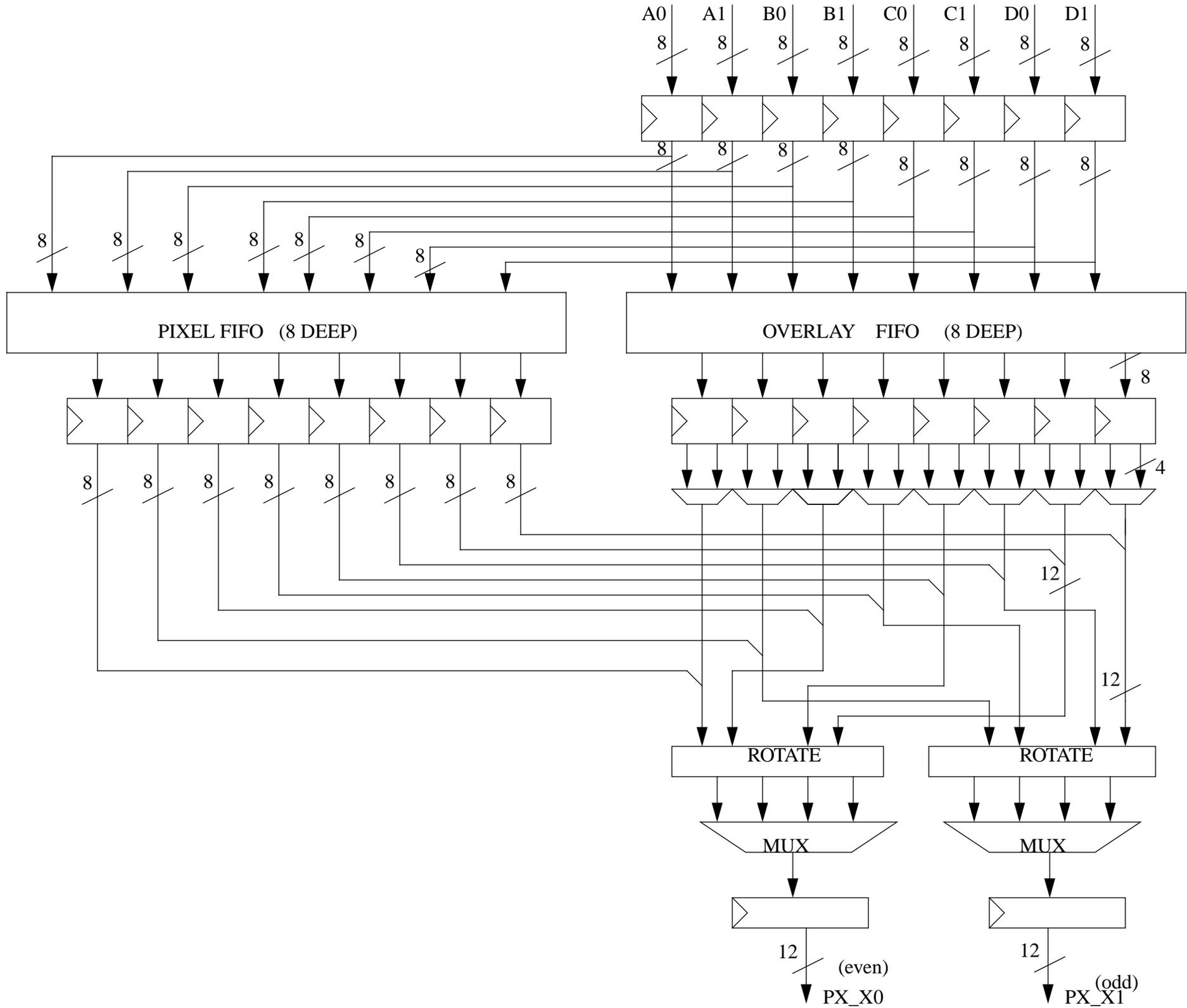
ing the fifos and merging the normal color and the overlay and sending out valid pixels to the XMAPs.
