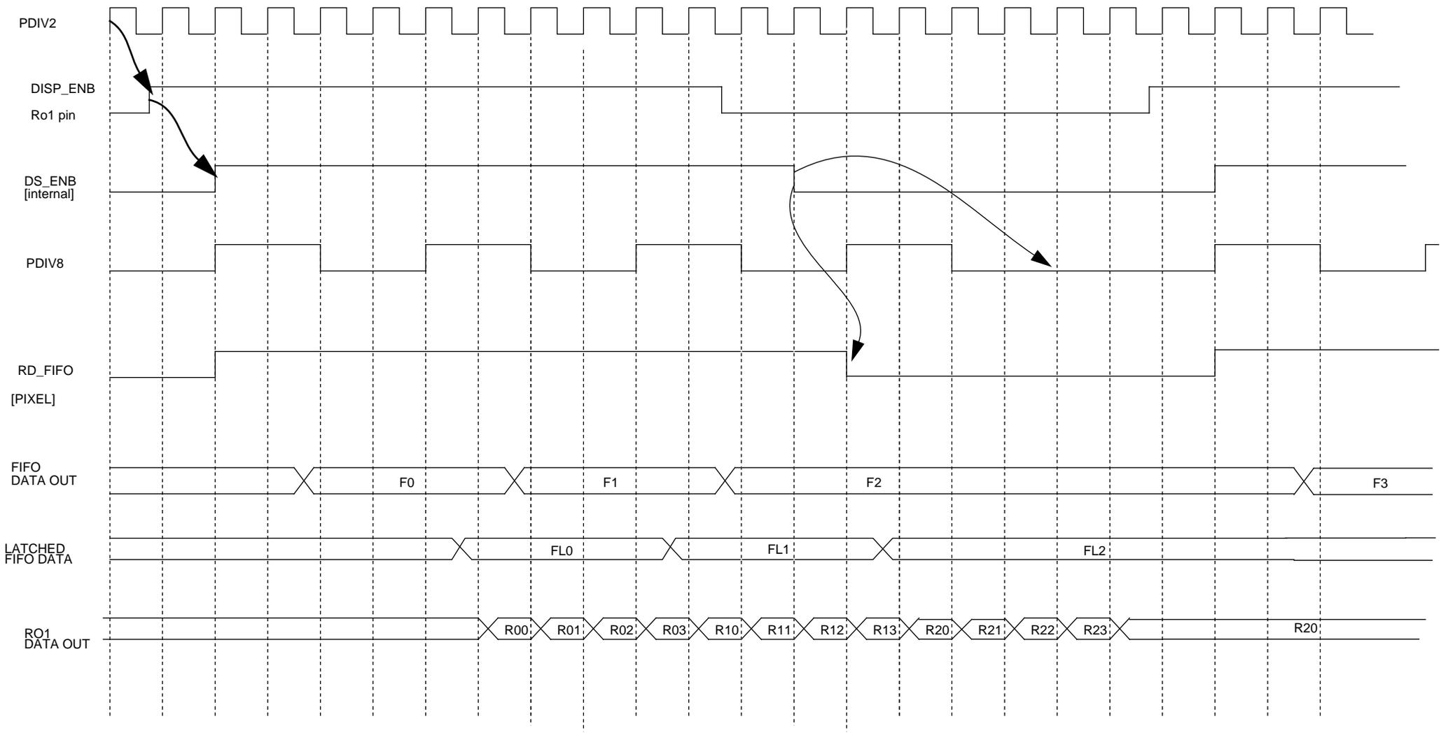
DISPLAY\_ENABLE FROM VC2, RO1 OUTPUTS DATA TO XMAP9 AT PIXDIV2 CLOCK
