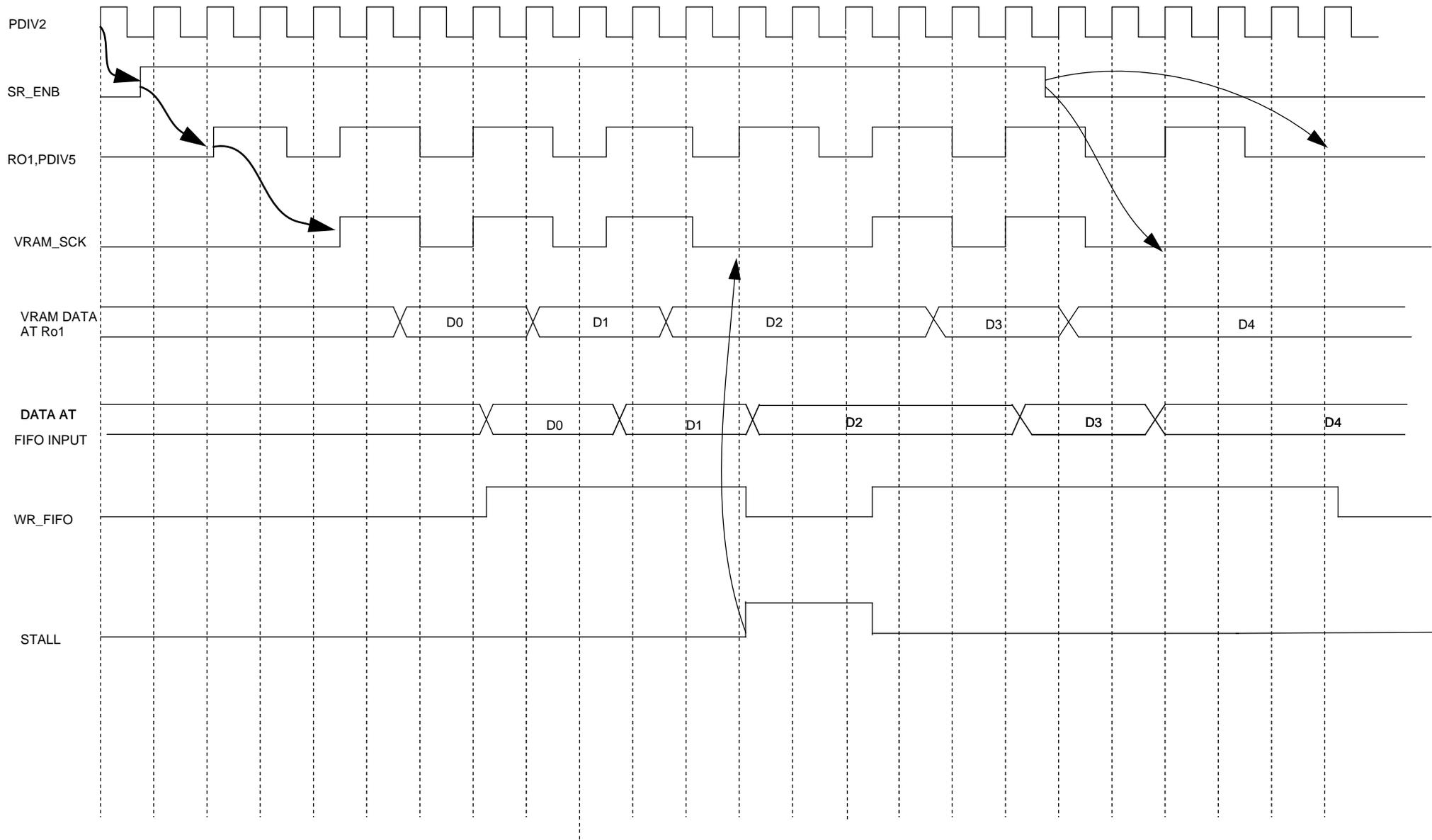
SERIAL ENABLE FROM VC2, RO1 LOADS DATA INTO FIFO
